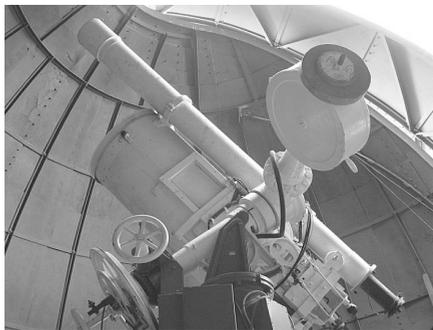
**Figure 8** The tall, slightly tapering tube of the 7-inch Merz, mounted as the guider for the 18-inch, before (top) and after (below) restoration.
